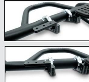
L-bracket in the **higher position**. This positions the pad above the top of most base handlebars.
